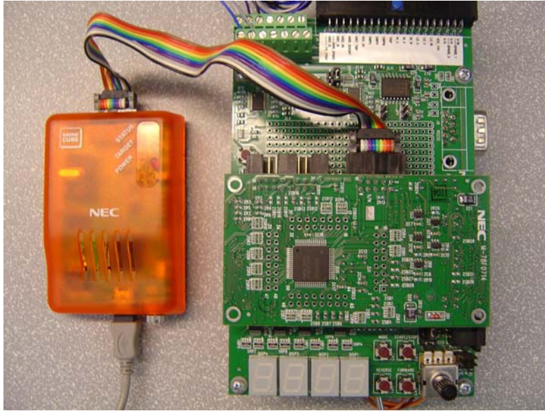
Figure 11. Debugging Environment Shown with QB-78K0MINI On-Chip Debugger
